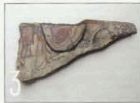
(Photo 3) I picked a slab with a good combination of pattern and color. An area of the chosen slab suggested a freeform shape, so I outlined the cabochon on the slab.
